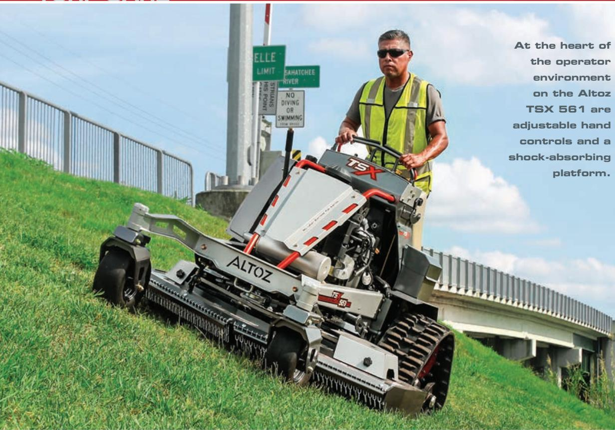
At the heart of the operator environment on the Altoz TSX 561 are adjustable hand controls and a shock-absorbing platform.
